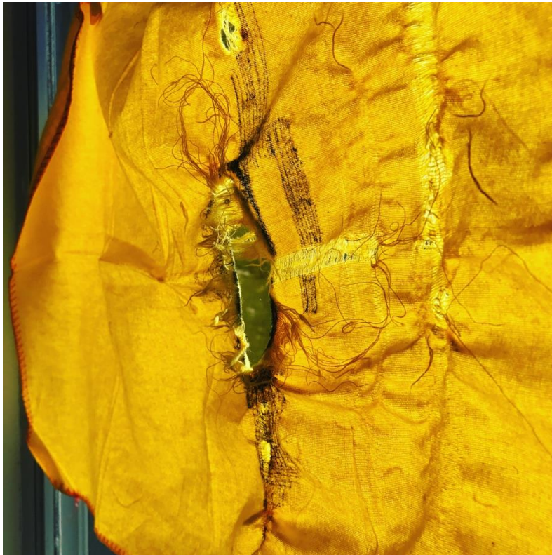
FIGURE 5A: DUSTER WITH HOLES MADE BY A NEEDLE
