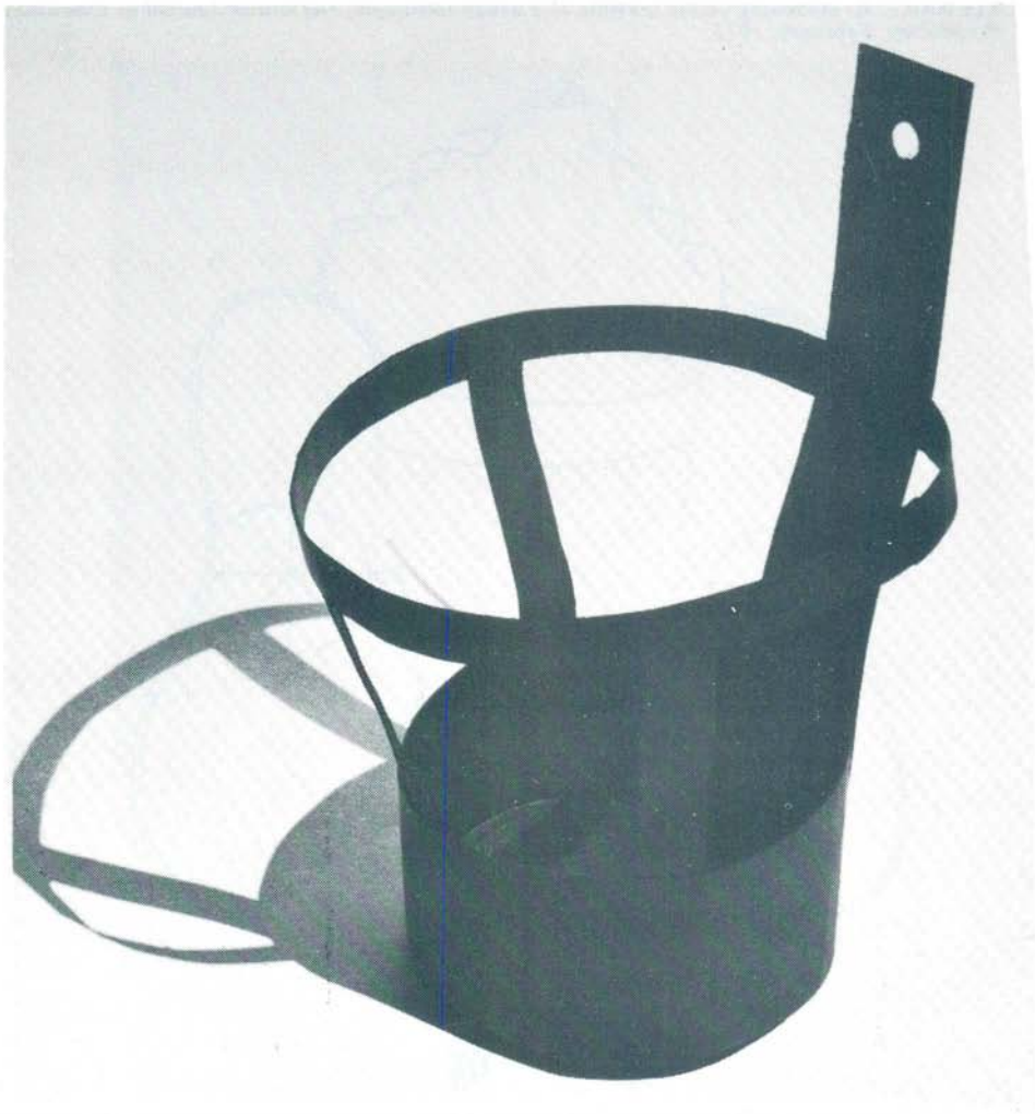
Fig. 1 A functionally effective and simple design for a wall plant-pot holder made in card by a first year grammar school pupil. The design is suitable for construction in mild steel strip and could be made by a schoolboy of reasonable ability.
