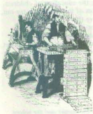
Preparing the paste-board cards for a Jacquard loom. From George Dodd 'The Textile Manufacturers of Great Britain, 1844'
