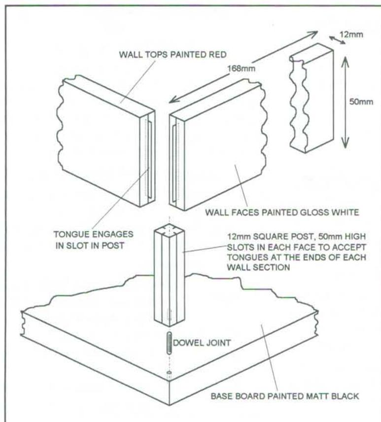
Figure 1: Basic maze construction
