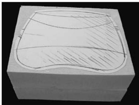
**Figure 6: Orthographic sketches bonded onto Styrofoam block.**
