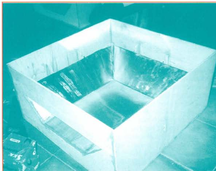
Figure 1 Cutting corners: measuring and sawing for two ovens at once. Figure 2 The oven interior, showing the aluminium before it is sprayed.
