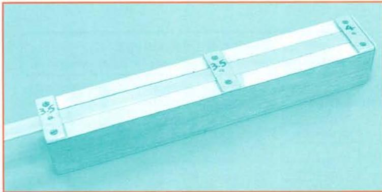
Figure 4: Jig for marking and drilling chassis
