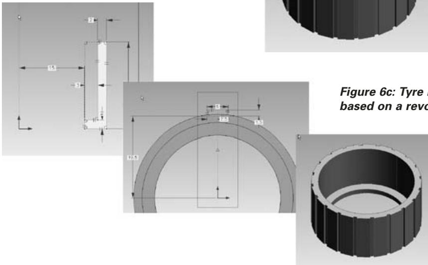
*Figure 6c: Tyre modelling approach based on a revolved X-section*
