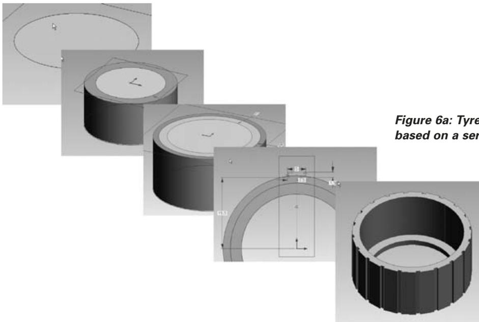
**Figure 6a: Tyre modelling approach based on a series of 'extrusions'**
