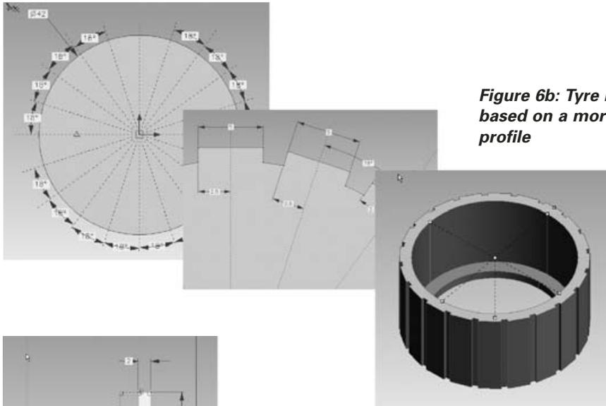
*Figure 6b: Tyre modelling approach based on a more complex sketched profile*
