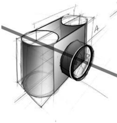
At this stage in the production of the sketch, crating and primitives have been employed to describe the geometry and proportions of the camera.
