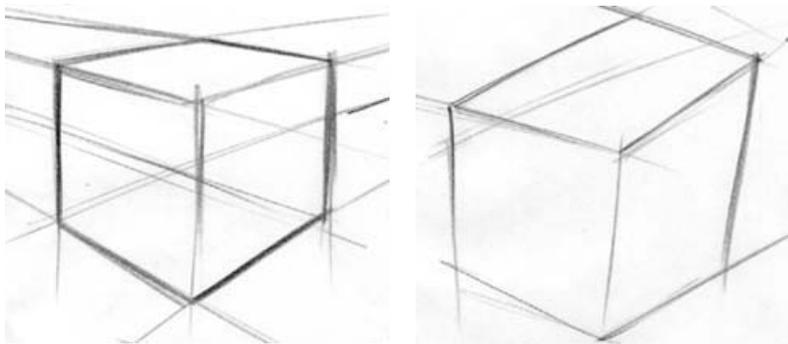
Figure 4. Shows a cube sketched using freehand two point perspective on the left and an example of common errors on the right.
