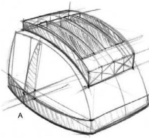
**iii) The toast slot area is added by projecting upwards from the top surface of the quadrant sketch. A section is used to define the curve on the product sides at A.**
