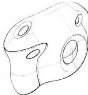
xiii) Tidy up line work and vary line thickness to describe form and component join lines etc.
